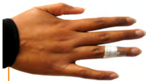
TLD Chip used for extremity dose measurement
