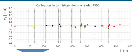
Extraction of drift values from a reader calibration history with linear interpolation/linear fit
